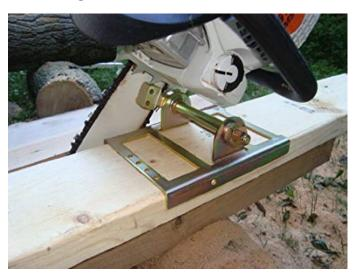
Advantages: Smaller chainsaw can be used to achieve similar cutting diameter to Alaskan, easy to fit, can saw vertical plane easily
