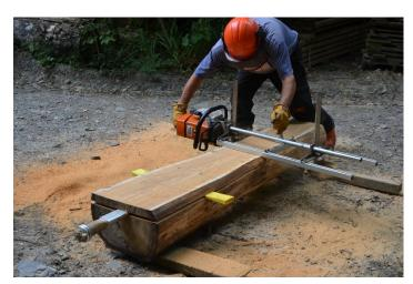
Advantages: Accuracy, good for sawing 'through and through' producing 'live edge' boards
