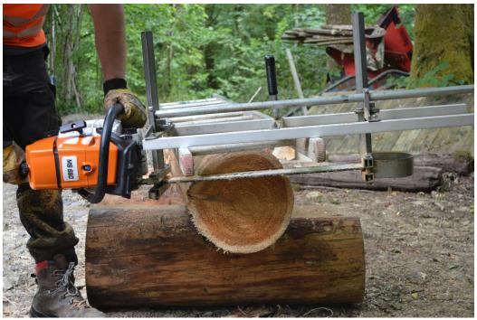
You need to keep a close eye on the four contact points between the guide rails where they rest on the straight edge, to ensure that they remain in contact. If one corner starts to rise the cut will not be straight, which will also affect subsequent cuts.
