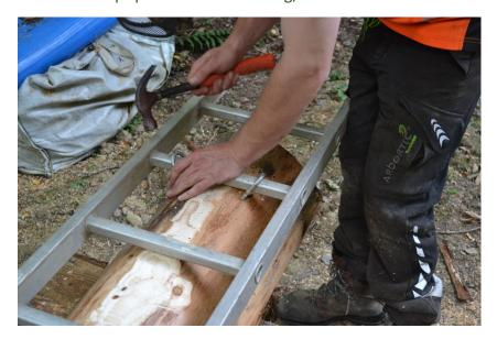
(iii) Measuring from the small diameter end of the log (the end with the wedges) the depth of the first cut is determined. You need the saw to comfortably **miss the staples** holding the ladder down, in this case 4/14 inches. If you wish to re-saw a further rail from the slabwood (eg: a 4" x 2") then allow for this now, optimising the recovery.
