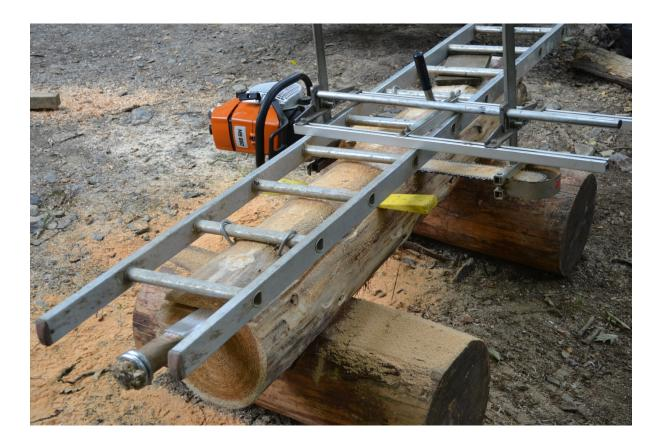
Proceed to the end of the cut, engage the chain break and remove the saw/mill. It is sensible to leave the saw running for a short while, rather than immediately switching off, to allow engine and other parts to cool down at the same rate.
