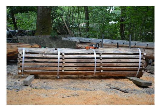
Boards will typically take about 6 months to air dry to around 20% moisture content. They can be further dried by a kilning process for indoor use.
