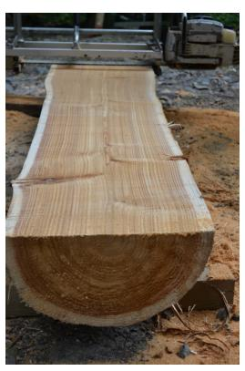
Here is a photo of a plank from the centre of a log, which was correctly set up for the first cut. The grain is exactly straight with the pith running along the whole length of the plank:
